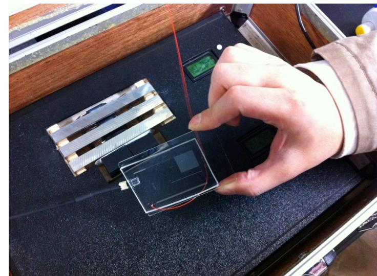
Printed electrode in RT-PCR flow chip for Flu virus detection
